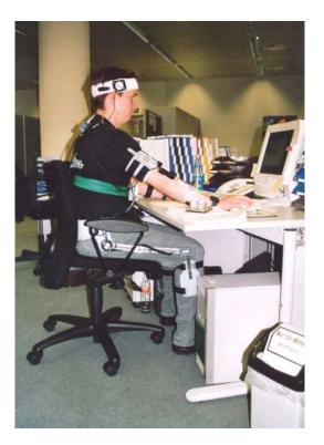
Posture measurements with the CUELA measurement system at a call-centre workplace
