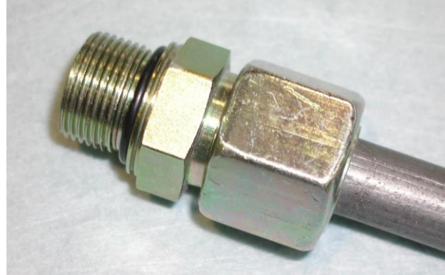
Figure 2: Example of a standardized unambiguous marking on stud ends according to DIN EN ISO 6149 with metric thread for pipe connections by means of notch (circumferential notch)
